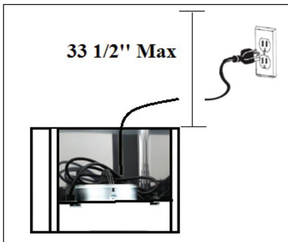
Place the outlet at a maximum distance of 33 1/2" from where the cord exits on the hood
