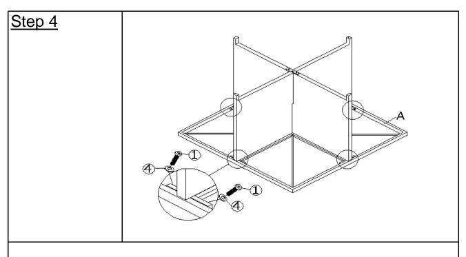
Attach Table Top(A) to Table Base using Bolts(1) and Flat Washer Rings(4) with Allen Key(7).
