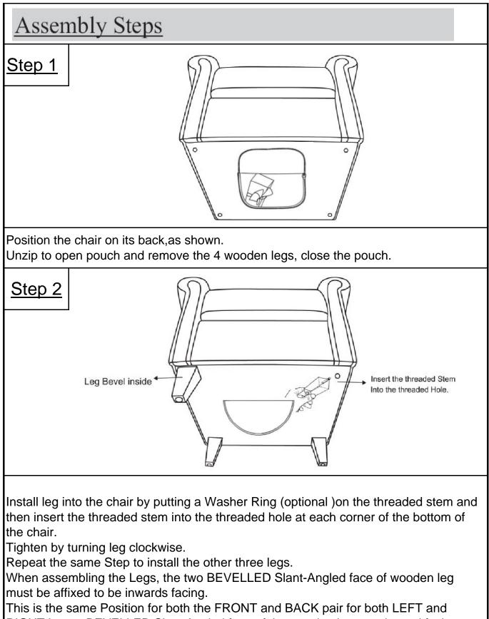
RIGHT Legs - BEVELLED Slant Angled face of the wooden legs are inward facing.
