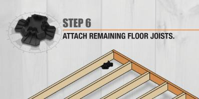
Position and attach the remaining floor joists to the trim boards using two 75mm (3 inches) counter sunk batten screws to attach the floor joist to the trim board.
