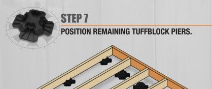
Using the frame as a guide, position the remaining TuffBlock piers directly beneath the frame. The blocks on the perimeter of the deck should be 300mm (12 inches) in from each end.
