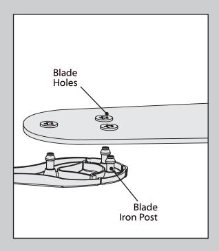
Align the three blade holes with the three blade iron posts. Squeeze the blade and the blade iron post together.
