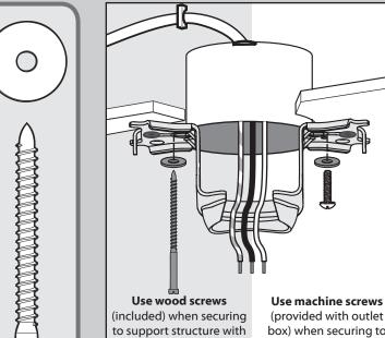
approved electrical outlet box. Drill 9/64" pilot holes in support structure to aid in securing ceiling bracket with hardware found in the  $\bigstar$  hardware bag.
