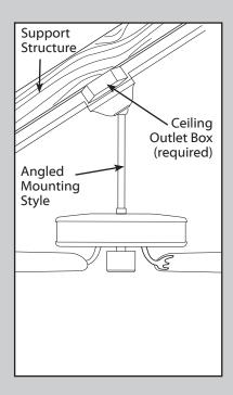
Use **Angled Mounting** to hang the fan from a vaulted or angled ceiling.
