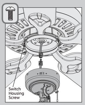
Partially install two of the switch housing screws found in the ≡ bag. Connect the plugs from the upper and lower switch housings. Make sure to line up the colored markings on the connectors.
