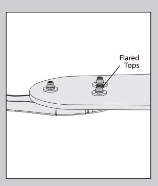
The flared tops of the blade iron posts will be fully visible above the blade when properly assembled.
