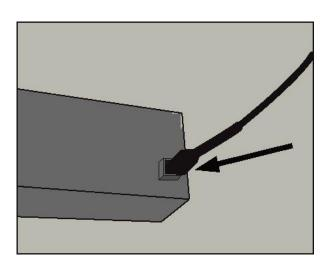
2. Make sure that the pilot housing is unobstructed. Clear any debris on top of the pilot housing and make sure there is no debris between the igniter pin, thermocouple and the burner tube.
