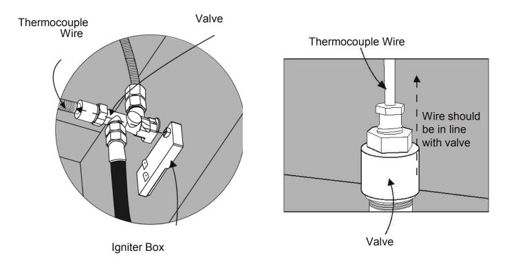
4. Make sure that the thermocouple wire is correctly positioned. The thermocouple wire should be in line with the valve.
