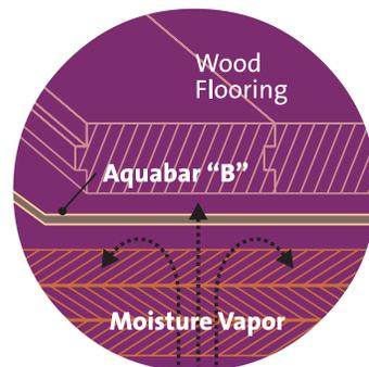
*Aquabar “B” helps slow moisture vapor originating below the wood floor system.*
