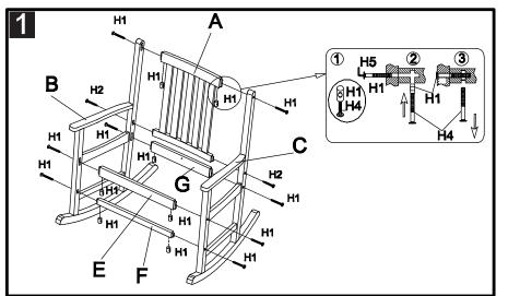
Step 1: attach the left side (C) and right side (B) to the back (A) by using Allen nut (H1) and Allen screw L (H2) as shown on the picture .Tighten with the Allen Key (H5). Make sure to tighten all positions before continue step 2.
