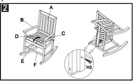
Step 2: put the seat (D) to the chair as shown on the picture and using the Allen screw S (H3) to fit .
