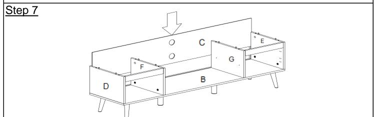
Insert the Back Panel(C) into the grooves on Left Side Panel(D), Right Side Panel(E) and Bottom Panel(B).
