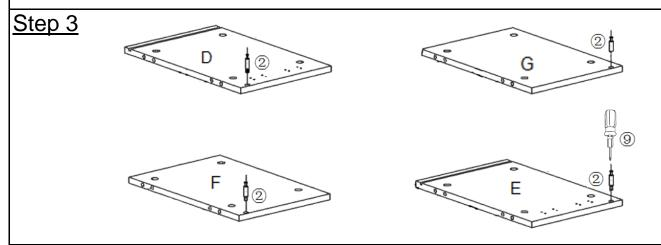
Attach Cam Bolts(②) to the mounting position on Left Side Panel(D),Left Stand Panel(F), Right Stand Panel(G) and Right Side Panel(E) with Screwdriver(③) as pictured.
