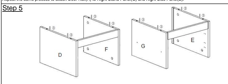
Insert Positioning Dowels(③) into mounting positions on Left Side Panel(D),Left Stand Panel(F), Right Stand Panel(G) and Right Side Panel(E) by hand as pictured above.
