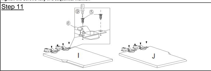
Attach Connectors(⑥) to the mounting position on Left Door Panel(I) using Screws(⑤) with Screwdriver(⑨) as pictured above.
