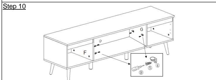
Attach Glass Clips(4) to Left Stand Panel(F) and Right Stand Panel(G) using Screws(5) with Screwdriver(9). **Tighten the Screws fully in a sequential manner.**
