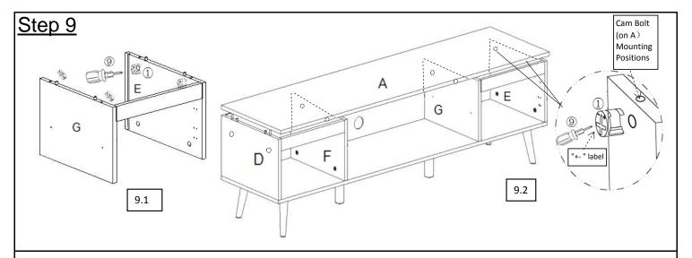
9.1:Insert Cam Locks(①) into the mounting positions on Left Stand Panel(F), Left Side Panel(D), Right Stand Panel(G) and Right Side Panel(E) with Screwdriver(⑨) as pictured.
