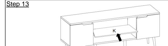
Carefully place Glass Panel(K) onto the suckers on Glass Clips(4).
