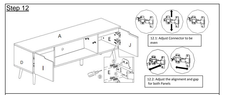
Attach Right Door Panel(J) with Connectors(6) to Right Side Panel(E) using Screws(5) with Screwdriver(9).
