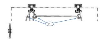
a) Tie one end of the pull cord to the left front bar of the awning, thread through left side pulley, then over closet right side pulley and down to the cleat and back up to open right pulley, tie the end of pull cord to the right and left side of the front bar. Draw all slack in pull cord towards cleat and tie off. (Shown Below)
