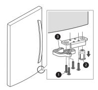
Reinstall the hinge pin brackets ①, screws
