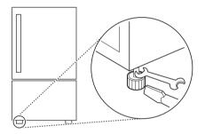
2 Open both doors and check to make sure that they close easily. If the doors do not close easily, tilt the refrigerator slightly more to the rear by turning both leveling legs to the left. It may take several more turns, and be sure to turn both leveling legs the same amount.
