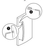
**3** Carefully loosen the plug buttons **3** with your fingers. The buttons can be unscrewed with the fingers by rotating them counter-clockwise and continuing until they loosen and fall out The buttons were installed without pressure, and for this reason, they can be unscrewed using your index finger, thumb or both. Install the plug buttons **4** on the left side.
