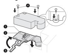
**15** Assemble the right hinge cap with the two screws.
