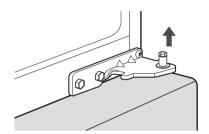
4 Remove the four screws ①, the hinge pin insert ② and the hinge pin brackets ③ from the bottom right side of the door.
