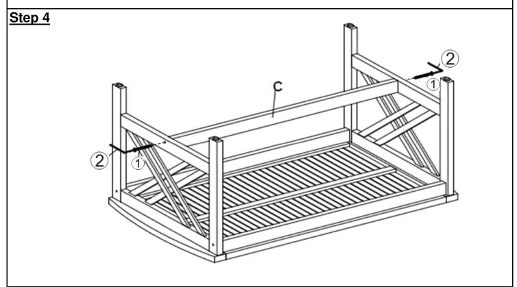
Affix Support Bar (C) to Leg Panels (B) by using Screws (1) and Allen Key (2). You may need to push the Leg Panels (B), outwards, slightly to attach the legs. **LOOSELY TIGHTEN THE SCREWS**, **up to 80%**.
