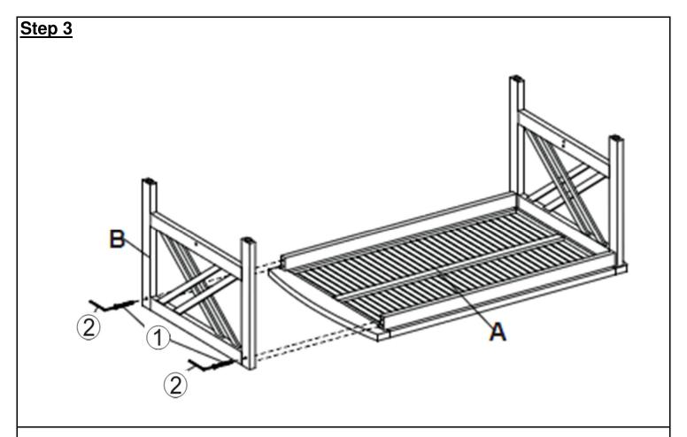
Repeat the same process to affix 2nd Leg Panel (B) to Table Top (A) by using Screws (1) and Allen Key (2) LOOSELY TIGHTEN THE SCREWS, up to 50%.
