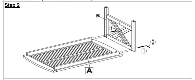
Position Table Top (A) and Leg Panel (B) as shown in picture above. Then affix 1st Leg Panel (B) to Table Top (A) by using Screws (1) and Allen Key (2) **LOSELY TIGHTEN THE SCREWS, up to 50%.**
