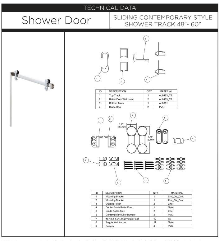
MATERIALS: INSTALLATION: UNIQUE FEATURE: Anodized Aluminum Excursions (Track) and Zinc Die Cast (Mounting Brackets). Bronze Finish is Powder Coated. Detailed Instructions and Hardware Included for Easy Installation. Constructed of Corrosion Resistant Anodized Alumninum.
