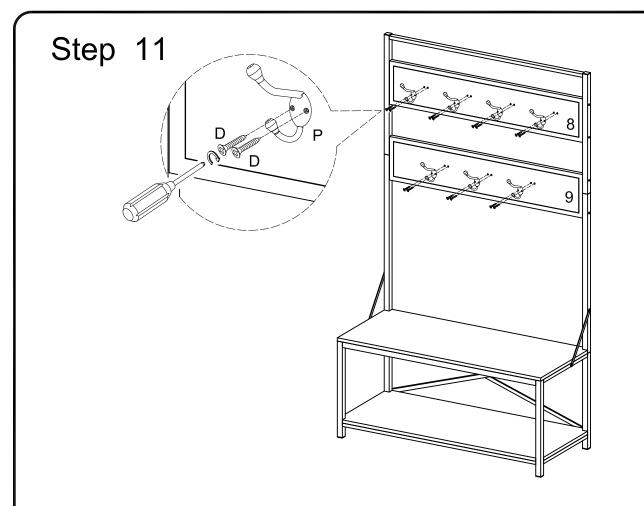
Secure hooks (P) to wood panels (8 & 9) using screws (D). Be careful not to over tighten.
