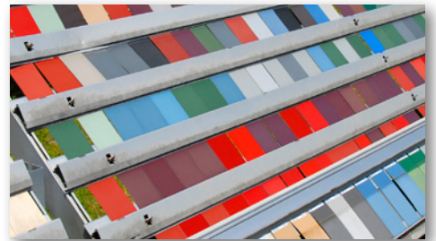
Test fences hold metal panels at a 45-degree angle in south Florida for maximum exposure.
