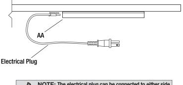
**NOTE:** The electrical plug can be connected to either side of the LED Fixture (AA).
