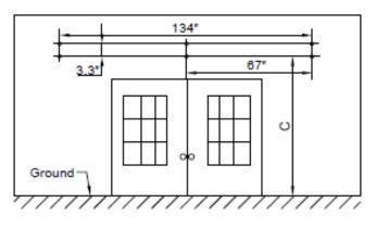
Note: When measuring to place the wall brackets, it is recommended to start measuring from the center brack outward.
