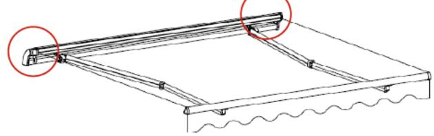
**IMPORTANT:** When installing the awning, verify that the elbow points on the arm stands are installed at the exact same location on each arm stand. This will ensure the awning will retract smoothly. If the awning jams or is not smooth when retracting, double check that the elbows are aligned correctly.
