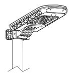
**Advice**: Ideal Pole Height: 6.5 - 13 feet; Ideal Pole Diameter: 1.5 - 2 inches. If multiple lights are purchased install between 25-40 feet apart for optimal light spread.
