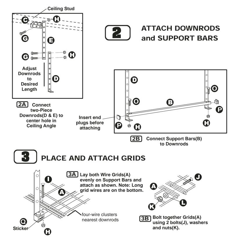
You have now completed the installation are ready to load your new HyLoft Storage Unit. **(Maximum 250 lbs. per 48" x 48" unit, evenly distributed)**. Place the sticker provided on a support bar for easy reference information.
