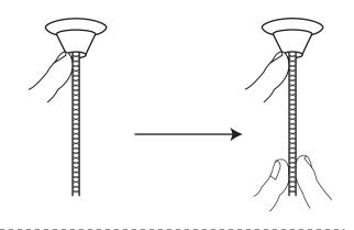
While holding the pin in place, simply pull down (or push up) on the cable. Repeat this for each cable to raise and lower the height of the fixture.
