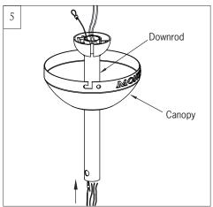
Place downrod over canopy. Thread lead wires and safety cable from motor assembly through downrod.
