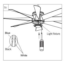
Connect white wire from fan to white wire from light fixture, and then connect blue wire from fan to black wire from light fixture.
