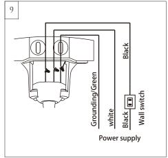
Make wiring connections using wire connectors provided as indicated above. Connect Black wire from fan to Black (Hot) wire from house. Connect White wire from Fan to White (Neutral) wire from house. Connect all green grounded wires to Grounded wire from House. Make sure that no filaments are outside of the wire connectors.
