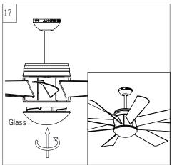
Attach glass to light pan by locating dimples in light pan with grooves on the glass and twist clockwise until tight.
