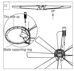
Flip the blade assembly over and install blade supporting ring onto the blades with screws provided.
