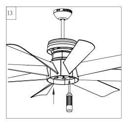
Lift blade assembly up. Aligning the preassembled setscrews on the flywheel and the screw holes on the motor and then install it onto the motor. Tighten screws securely.
