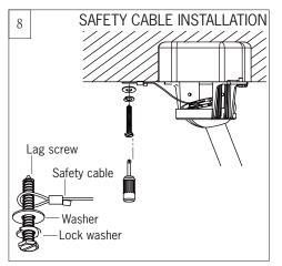
For Canadian installation and for USA fan and light kit combinations over 35 lbs, in both flush and downrod mode the safety cable must be installed into the house structure beams using 3" lag screws, washers and lock washers provided. Make sure that when the safety cable is fully extended the lead wires are longer than the cable and no stress is placed on the lead wires.
