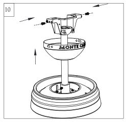
Partially loosen 2 of the set screws on mounting bracket corresponding to the slotted holes on the canopy upper ring. Remove the other 2 set screws. Save screws.
