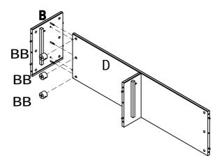
**7** Connect right side panel(C) to divider panel(D) with cam lock(BB) from step 6
