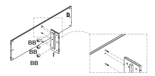
**6** Connect left side panel(B) to divider panel(D) with cam lock(BB) from step 5
