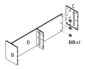
${f 8}$  Connect layer box(H) with cam lock(BB) from step 7 as shown
