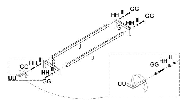
**10** Use allen key(UU) to tighten step 8 and step 9 with screw(GG) and washer(HH&II)
