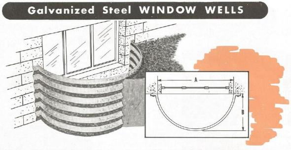
Vestal Window Wells provide light, ventilation and positive protection to basement windows located below ground level. Simply set in place and fasten to masonry foundation with masonry nails. Eliminates costly concrete forming.
