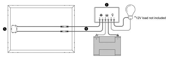
Remove the panel covering. In good sunlight, the charge controller's • "BAT %" should increase to 100%. Once the battery is fully charged and the controller is set to "LOAD ON," the system will provide power through the load control output or through the two USB ports. If an inverter is added to the system, it must be connected to the battery bank, and not to the charge controller.
