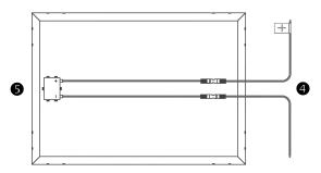
Connect the bare wire end of the positive cable **4** to the "SOLAR +" input of the charge controller **4**. Connect the negative bare end to the "SOLAR -" input. Now, you can mount the PWM-165 to an indoor wall or within a NEMA-3R rated enclosure.
