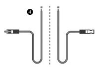
Connect the MC4 ends of the halved cable 4 to the compatible MC4 ends of the solar panel 5 cables.
