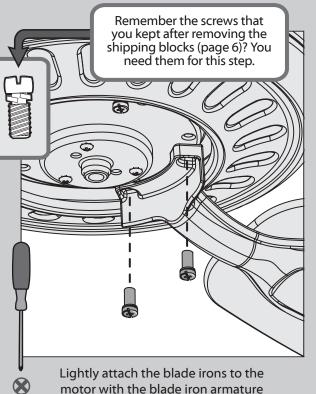
notor with the blade iron armature screws, then securely tighten after both screws are attached.
