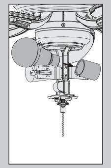
Install the included LED bulbs into the sockets. When necessary, replace with bulbs of same wattage.
