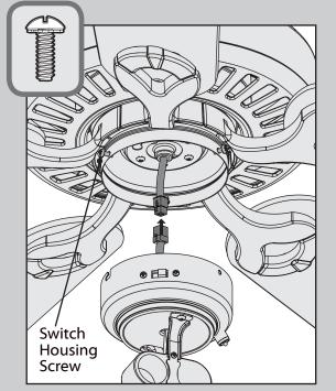
Partially install two of the switch housing screws found in the ≡ hardware bag. Connect the plugs from the upper and lower switch housings. Make sure to line up the colored markings on the connectors.
