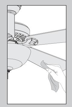
**Cleaning the fan** - use soft brushes or cloths to prevent scratching. Cleaning products may damage the finishes.
