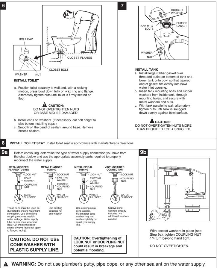
connection to this tank. If the connection leaks after hand tightening, replace the supply line. If the connection continues to leak with the new supply line, replace the fill valve.
