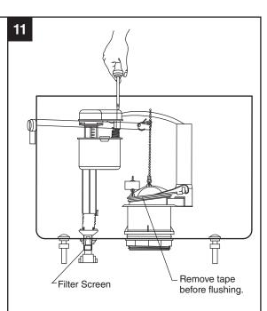
Adjust tank water level to the proper marked waterline by rotating threaded rod clockwise to raise water level or counterclockwise to lower water level.
