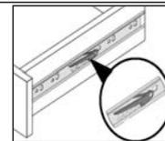
press down the pin on this side & press up the one on another side to pull out the drawer box.
