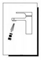
4.After installing faucet, remove aerator assembly and open the hot and cold water supplies. Check for leaks.Turn on faucet handle for one minute to flush debris from faucet.Close the handle and re-assemble the aerator.
