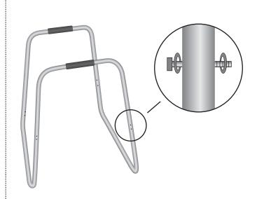
Insert the **5" screws** into the **8 holes** making sure there is a **washer** one each side of the screw as shown.
