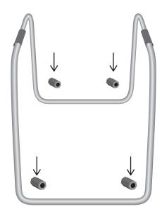
Attach the **4 rubber feet** to each of the legs. Your DIPSTAND is now completely assembled!
