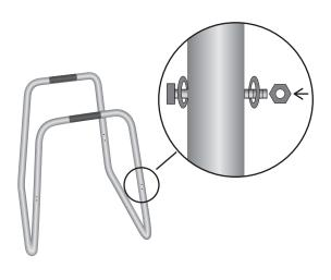
Use wrench and Allen key to secure the **8 nuts** onto all **8 screws**.
