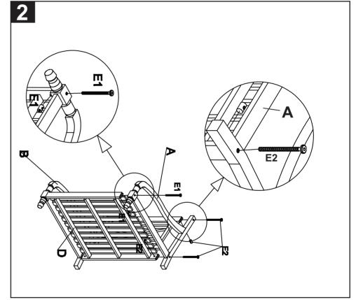
Step1: attach the right side (B) and the back(C) to the seat (D) as shown on the picture by using the Allen bolt (E1) and (E2).Tighten with the Allen key (E4).
