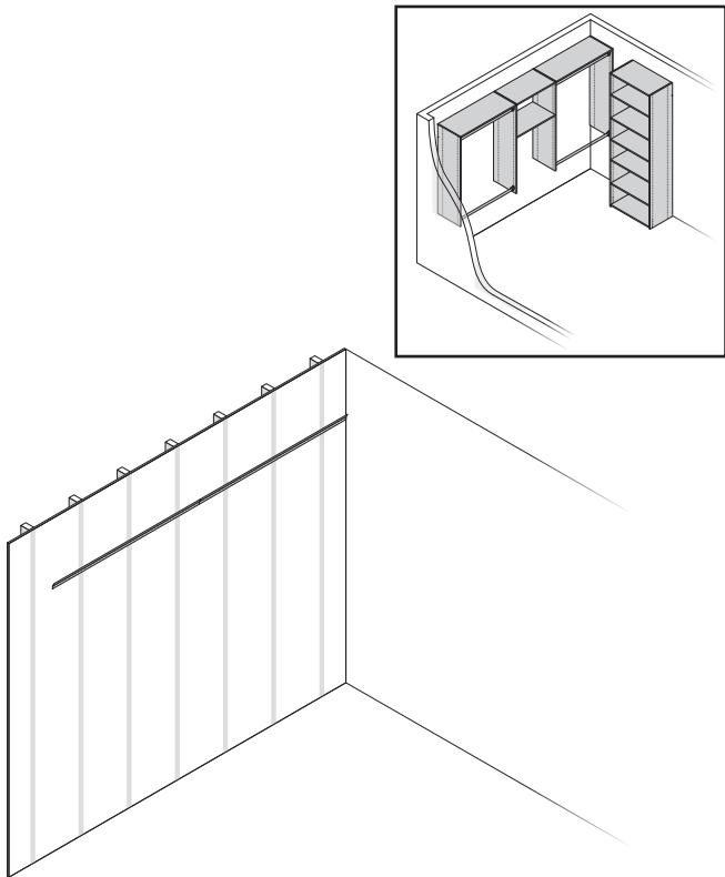
5 When installing the adjacent wall kit, start the track 24" from the wall. Verticals should be installed at 26" in order to provide 2" of track overhang.
