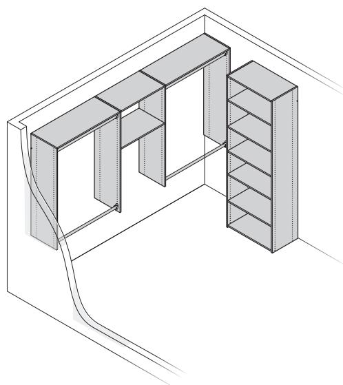
**1** Decide where to locate the top of the vertical panel. Mark a hang line for the track 8.5" down from the top of the vertical panel.
