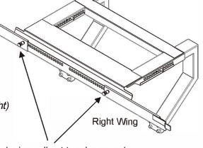
Lock pins pull out to release and push in to lock into slotted holes.
