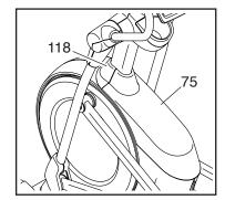
**See assembly step 15 on page 14.** Remove the Right Leg Outer and Inner Covers (69, 83).
