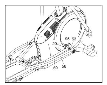
See EXPLODED DRAWING C on page 35. Identify the Left and Right Shields (73, 74). Remove the M4 x 19mm Tek Screws (5), the M4 x 19mm Screws (124), and the M4 x 48mm Screw (107) from the Left and Right Shields; make sure to note the location of each size of Screw. Then, remove the Right Shield.
