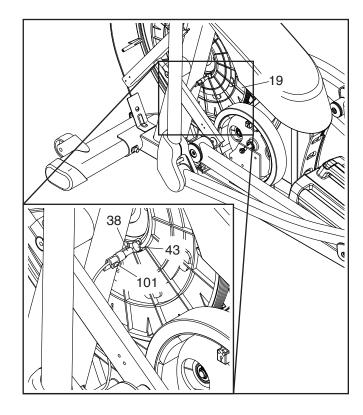
Next, slightly loosen the indicated M4 x 16mm Screw (101). Slide the Reed Switch (38) slightly closer to or away from the Magnet (43), and then retighten the Screw.
