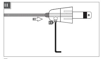
**II** Firmly tighten the set screw on the conical connector.
