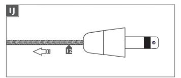
Pull the coaxial cable toward the fixture to smooth the wrinkles.
