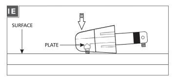
**6** Tap the conical connector on a hard surface with the set screw facing down, so the plate inside drops into place.
