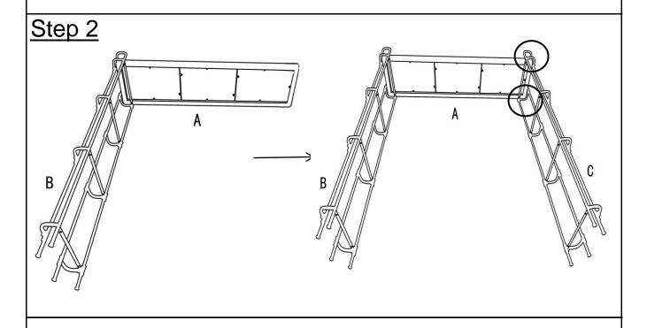
Attach Wooden Shelf(A) to Right Leg Frame(C) using Bolt(3) with Allen Key(4). **Only Loosely Tighten.**
