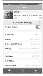
The timer's Settings screen contains everything else needed to fully control your irrigation system. It can be reached by selecting the Controller Settings button on the bottom of the screen.
