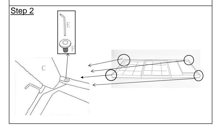
Attach Front and Back Leg((C) to the Lounge(A) using Bolt(F) with Allen Key(E). **Do not tighten Bolts**.
