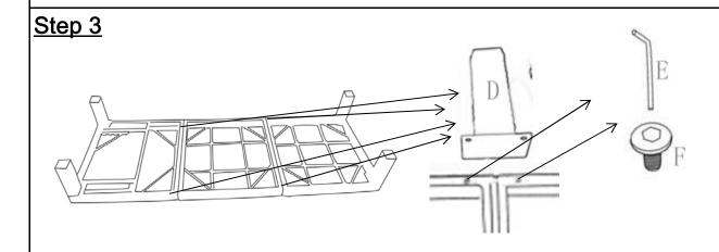
Attach Middle Leg((D) to the Seat Panel(A) using Bolt(F) with Allen Key(E). Now, in asequential manner, proceed to fully tighten all Bolts at all joints.
