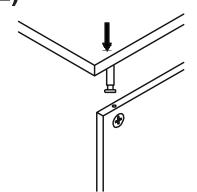
Insert the cam lock bolt into the pre-drilled hole above the cam connector.
