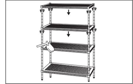
6: Repeat the step(2) and the step(3) to assemble the 3rd and the 4th perforated steel shelf as the photo. Then pushing firmly down on every perforated steel shelf at corners by rubber mallet to secure the perforated steel shelf in a place over the plastic clips.
