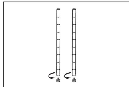
1: Screw the adjustable feet to the one-piece pole.
