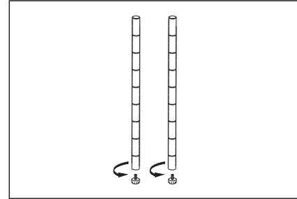
1: Screw the adjustable feet to the lower poles.
