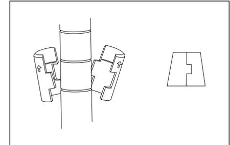
2: Snap the plastic clips into the pole groove of four lower poles at the same position.
