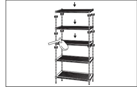
6: Repeat the step(2) and the step(3) to assemble the 3rd and the 4th&5th perforated steel shelf as the photo. Then pushing firmly down on every perforated steel shelf at corners by rubber mallet to secure the perforated steel shelf in a place over the plastic clips.
