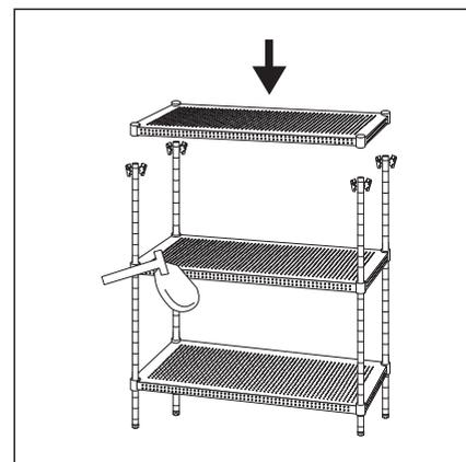
6: Repeat the step(2) and the step(3) to assemble the 3rd perforated steel shelf as the photo. Then pushing firmly down on every perforated steel shelf at corners by rubber mallet to secure the perforated steel shelf in a place over the plastic clips.
