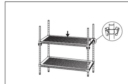
4: Repeat the step (2) and the step (3) to assemble the 2nd perforated steel shelf (A) as the photo.
