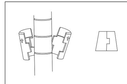
2: Snap the plastic clips into the pole groove of four one-piece pole at the same position.
