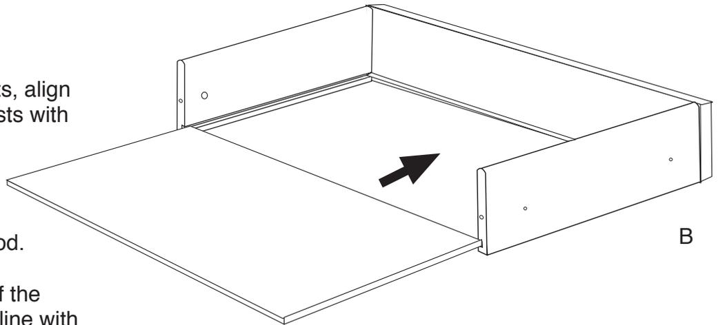
C. Take two (2) Bastion Posts, align the threaded ends of the Posts with the post holes located near the ends of the inside Drawer Front. Tighten Posts down until the solid shaft of the Post hits the wood. Back Post out until the hole/screwdriver slot in the end of the Post is parallel and in direct line with the long edges of the Drawer Front.
