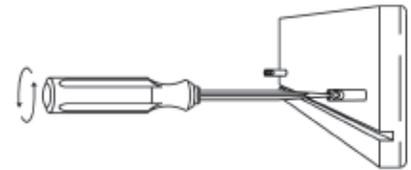
D. Insert the B-Nuts into the nut access holes on the inside of the Drawer Sides with the threaded end facing out. Take the Drawer Front and carefully insert the Posts into the ends of the Brace Sides, through the sides of the B-Nut until seated. Push Nut snugly against the wood in the nut access hole toward the Drawer Front. Hole should be slightly off-center toward the Drawer Front. Insert the Set Screw and tighten down. The Drawer Sides should be tight against the Drawer Front.
