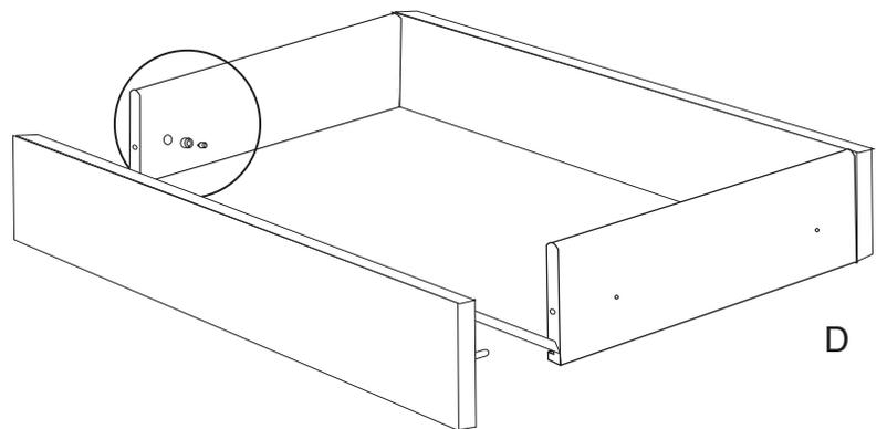
E. Attach the Drawer Glides (left and Right) to the Drawer Sides using two 7/16" #6 Pan Head Screws per glide. Open end of glide goes toward the back of the drawer. (DO NOT INSERT DRAWER INTO CABINET AT THIS TIME). Glide is almost flush with the back of the drawer front.
