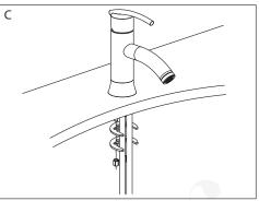
C. Insert the rubber washer, metal washer, and secure the faucet with the mounting nut.
