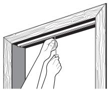
Do not fully tighten. (Tape may be used to hold the track in place while you mark and drill.)
