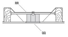
To hang your fan where there is an existing fixture but no ceiling joist, you may need an installation hanger bar (RR) (not included) as shown above.
