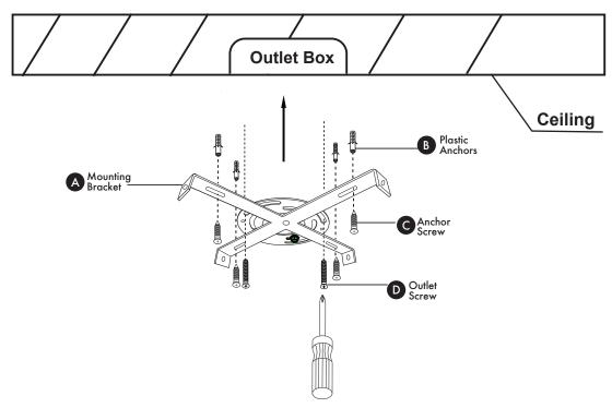
Attach mounting bracket (A) to outlet box with oulet screws (D). Screw anchor screws (C) into plastic anchors (B) to secure mounting bracket (A).
