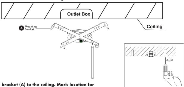
Raise mounting bracket (A) to the ceiling. Mark location for the plastic anchors (B). Drill holes for plastic anchors (B). Insert plastic anchors (B) into hole.
