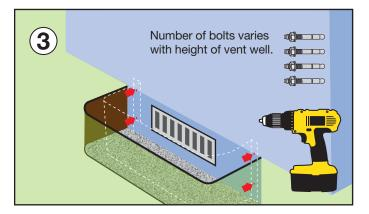
Drill holes to receive the ancnor poits, then secure the vent well to the foundation using anchor bolts and optional flat washers.
