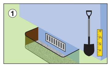
Pre-fill hole with at least 4" of gravel or drain rock to promote drainage. If flooding is a concern, connection to a perimeter drainage system might be required.
