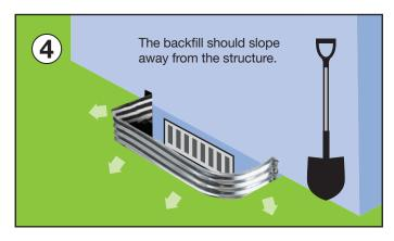
Add gravel to the well bringing the level up to 2" below the bottom of the vent opening. Backfill the area between the vent well and the hole.
