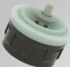
Although filtering of sediments in the dome is a better solution than the wire mesh aerator for areas with low debris/sediment in the water, the dome screen can quickly become clogged. In construction sites where the main water system is periodically interrupted for maintenance "flushing", this can become a problem.
