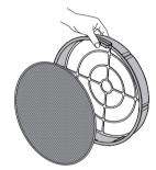
6. After cleaning or replacing filters, assemble the filters in the set in the reverse order from removing them. Be sure to insert the filters behind the bottom tab and align the filter handles at the top of the product.
