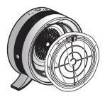
4. Insert the filter behind the bottom tab and snap it into place at the top.
