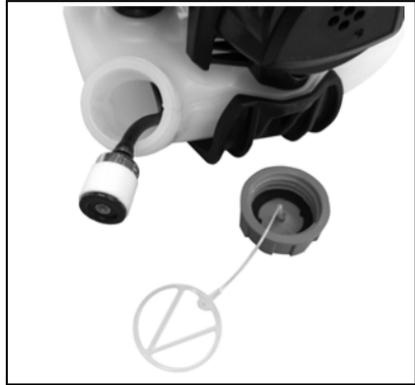
*Do not damage fuel line while removing fuel filter from tank.*
