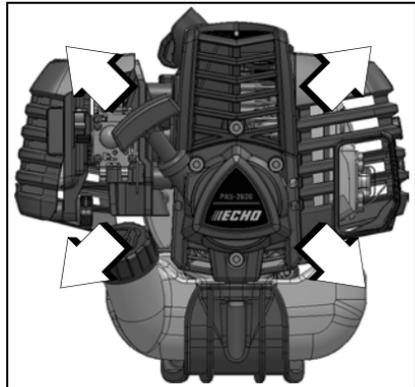
Removal of cooling passage blockages or cleaning of cooling fins is considered "Normal Maintenance." Any failure attributed to lack of maintenance is not warranted.
