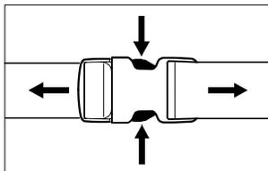
**D** Squeeze the hooks to open the quick-release fastener.
