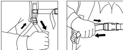
**A** Once the blower is properly fitted on your back, pull the ends of the straps downward to tighten the harness. Connect the horizontal chest strap, and pull the end of the strap to tighten.
