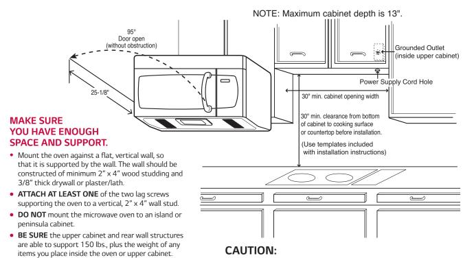
Before you begin installing the oven, PLACE A PIECE OF THE CARTON OR OTHER HEAVY MATERIAL (a blanket) over the countertop or cooktop to protect it. Do not use a plastic cover. Failure to protect these surfaces could result in property
